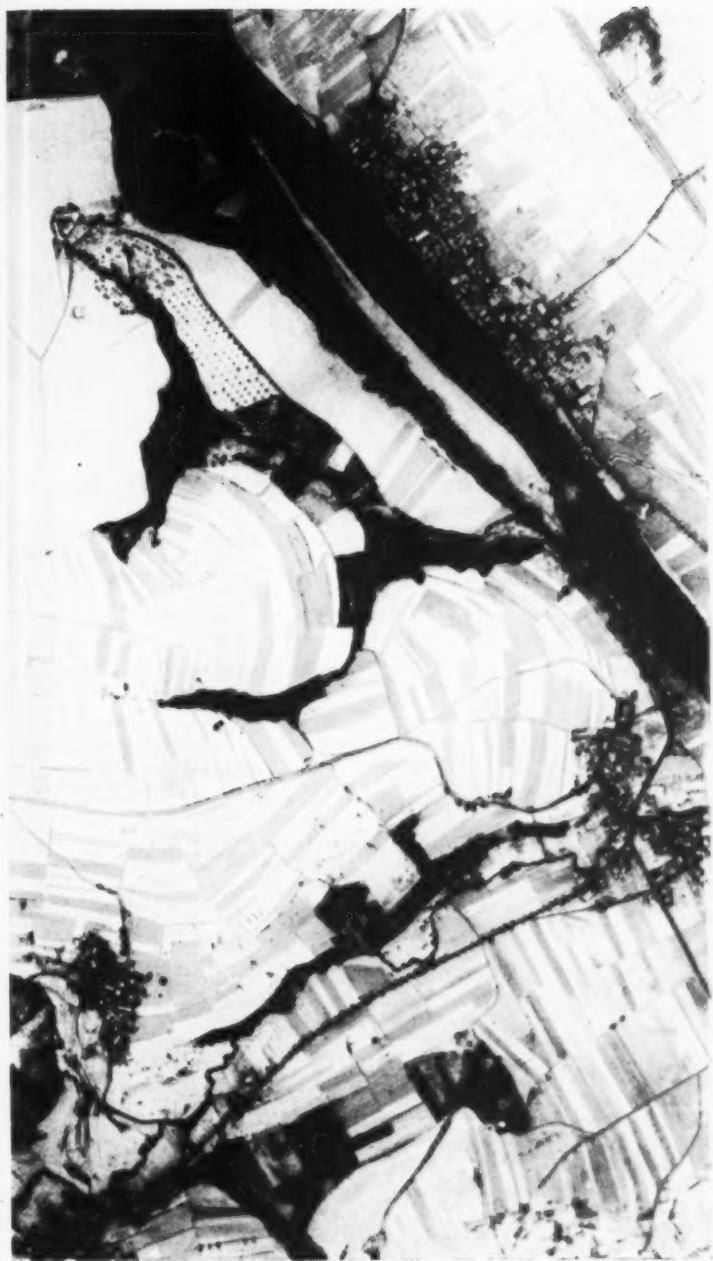
AIR PHOTOGRAPH OF GROUND COVERED BY MAP OPPOSITE: THE CULTIVATION LINES (WHICH HAVE BEEN STRENGTHENED IN THE REPRODUCTION) SHOW THE TREND OF THE CONTOURS
